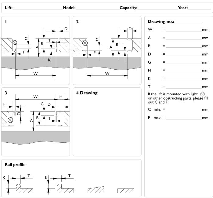
**PLEASE NOTE:** It is the customer's responsibility that the given measures are correct and sufficient. **N.b. EN I 493:1998** the capacity of the jacking beam cannot exceed 0,66 x the capacity of the lift. (A 2 t jacking beam on a 3 t lift is okay - but not a 2,6 t).
