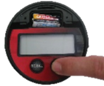
Step 3: Insert the new battery and press the RESET button to check the function of the register
