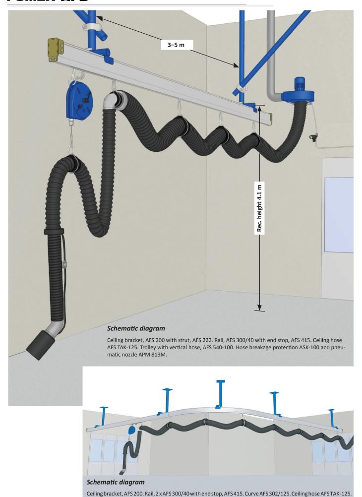
Trolley with vertical hose, AFS 565-100. Hose breakage protection ASK-100 and pneumatic nozzle APM 813M.
