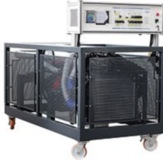
Educational Truck Diesel engine with PLD system
