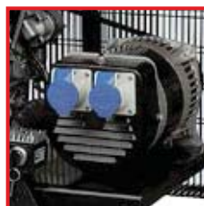
Generator with electricity plug at 230 volt
