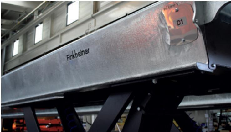
To increase the life expectancy of a lift in a wash hall, we treat the lift with a special surface treatment. Platforms and scissor elements are hot-galvanised, the control box and covers are made of stainless steel, for example.
