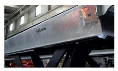
To increase the life expectancy of a lift in a wash hall, we treat the lift with a special surface treatment. Platforms and scissor elements are hot-galvanised, the control box and covers are made of stainless steel, for example.
