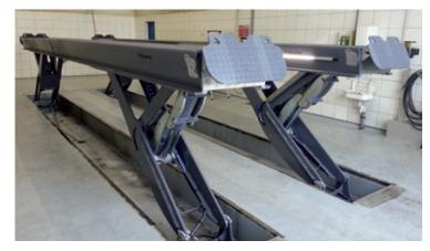
The DUROPLEX coating contains a surface treatment for platforms, ramps, scissor elements and floor plates in addition to the hot galvanisation. We achieve corrosivity class C5 I by bead blasting and applying several coatings.
