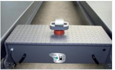
Electro-hydraulic jacking beam
