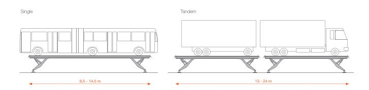
The platform lift HDS® is suitable for all vehicles, from compact forklifts to complete truck and trailer. For long vehicles you can combine two single lifts to a tandem lift. Each lift can then still be used as a separate single lift. Flexibility, which creates many different possible applications.
