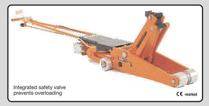
The jack, which is ruggedly dimensioned and robust despite its low initial height, is equipped with double internally ground and hard chromed lifting cylinders with ground and hard chromed piston rods.
