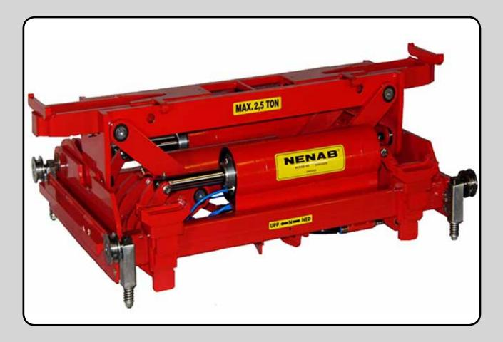
The lift is intended to be used for lifting cars, checking and repair of the wheel suspension, steering control, wheel bearings, tires and more.
