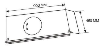
The plate can take a maximum load of 1250 kg (axle load of 2500 kg), and has a weight of 35 kg each. The plate can move 40 mm forth and back, and 40 mm to both sides. The height is 40 mm. The turn table can rotate 360°. The plates are supplied in pairs of two. Ordering no. 100701.
