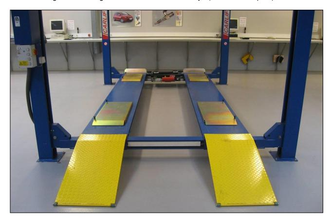
The front plate is a unique design, where the whole plate can turn, and the turn table, inside the plate, turns too. The space behind the round turn table is used for rolling back compensation.
