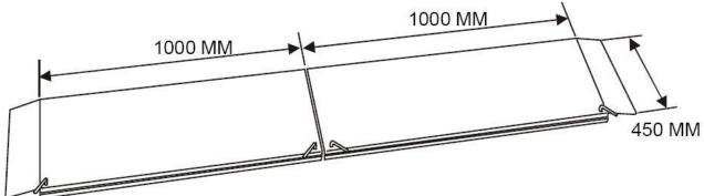
The plate can take a maximum load of 1250 kg (axle load of 2500 kg), and has a weight of 80 kg each (2x40 kg for each side). The plate can move 2 mm forth and back, and 40 mm to both sides. The height is 40 mm. The plate can rotate 6<sup>0</sup> in and out. The plates are supplied in pairs, each two plates. Ordering no. 100703.
