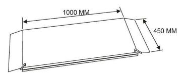
The plate can take a maximum load of 1250 kg (axle load of 2500 kg), and has a weight of 40 kg each. The plate can move 2 mm forth and back, and 40 mm to both sides. The plate can rotate 6<sup>0</sup> in and out. The plates are supplied in pairs of two.
