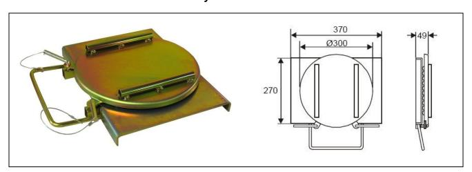
Our rear turn table is equipped with safety anti-rolling bars, to avoid the vehicle of rolling off the turn tables. This feature enables an accurate measurement of the turning angles.
