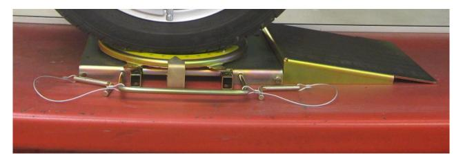
The drive on turn tables can be used for non-compensation wheel adapters, such as BMW, Mercedes, Porsche aso. Aligning a vehicle with drive on turn tables is fast and ensures the correct ride height of the vehicle, and the suspension in driving condition. The ramps can be supplied in combination with the turn tables 100104, 100124, and 100124L.
