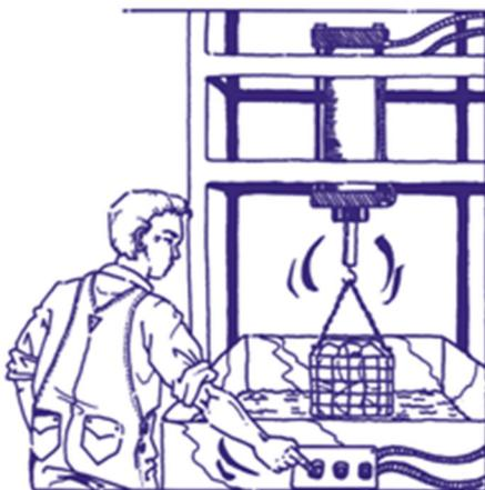
In a car factory, metal parts are dipped in solvent to remove grease. Could a single acting cylinder raise and lower the basket?
