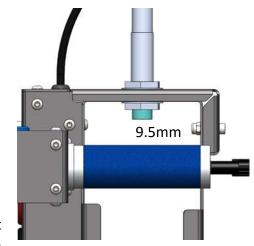
Adjust the height of the inductive sensor to the conveyor so that it is roughly '9.5'mm distance away from the conveyor belt.
