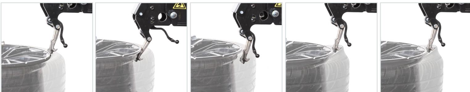
The latest generation new super-automatic tyre changer for car wheels, SUVs and commercial vehicles up to 30". The new dynamic tool, thanks to its geometry, creates an angle between rim and bead that allows considerable reduction of bending on the tyre and of contact with the rim. The reinforced structure, the super-performing clamping, ergonomics, and intuitive controls ensure operational speed, effortless work and make it usable at 360°
