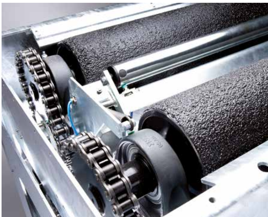
Strong mechanics: weather-resistant hot-dip galvanization, steel chains
