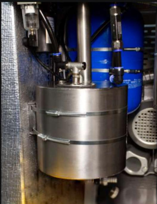
The automatic detergent dispenser is a feature designed to simplify the cleaning process in DPF machines. Traditionally, it is accepted to add 200 ml of cleaning fluid concentrate to the machine's tank for each DPF filter before cleaning, which typically involves manual allocation of the detergent. Aiming to facilitate this process, Otomatic introduced an automatic detergent dosing function during the wet cleaning process without the operator's intervention.
