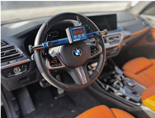
Digital Bluetooth steering level gauge in the scope of deliveries Order number: 1 693 770 619
